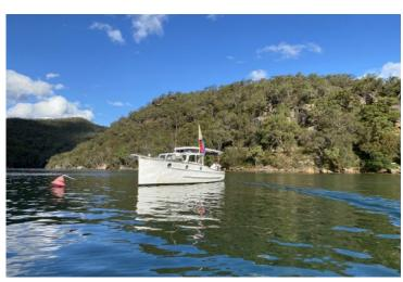
The hull is traditional planked Oregon timber, with good hull protection and integrity offered with the extended berthing strakes. The deck and cockpit are fiberglass ply, the foredeck and aft deck are beautifully laid with oiled Beech timber. The interior joinery is very original with 2 x full berths with custom mattresses. There is a small private toilet area fwd. The galley is basic with a stainless sink and small bench.
